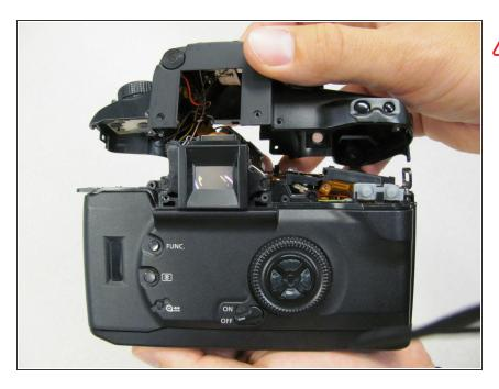
Separating the top panel too far can damage the connecting wiring.
