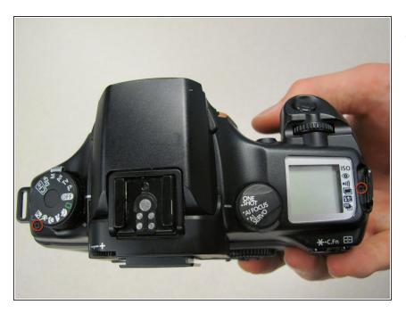
Remove two 4.75 mm screws from top of camera.
