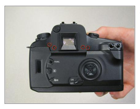
Remove four 4.3 mm screws from back of camera.
