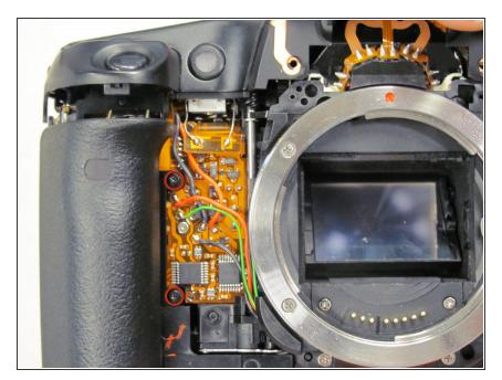
Remove two 5.5 mm screws from front of camera.
