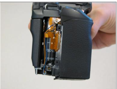
Slide panel toward bottom of camera to remove.
