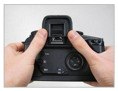
Remove outer eyepiece by sliding it upwards.
