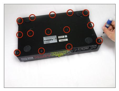
Flip the device over. Using a Philips #2 screw driver, remove the fourteen 10.3 mm black screws holding the back panel in place.
