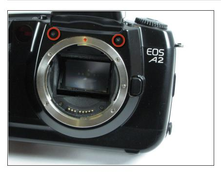
Remove the two 6.4mm screws above the lens aperture using a phillips #00 screw driver.
