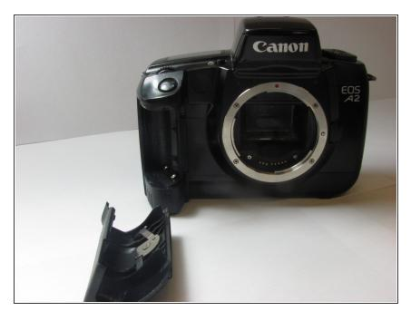
Remove the battery from inside the battery housing and set the cover aside.
