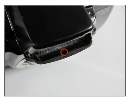
Remove the 6.4mm screw from the inside of the flash bezel.
