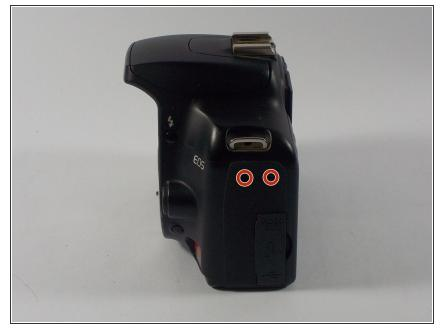
Remove the two 4.5mm (.18in) long black screws from the side cover using a #00 Phillips screwdriver.
