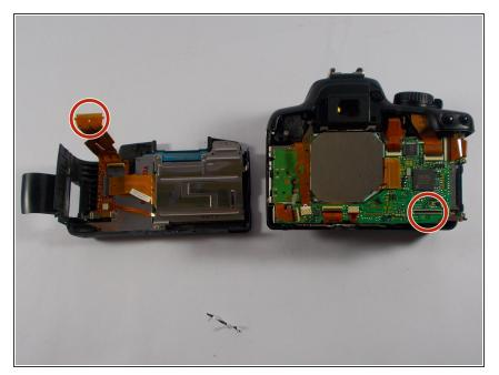
Once you have detached the back cover, use a pair of tweezers to lightly pull on strap found connecting the back cover to the camera.
