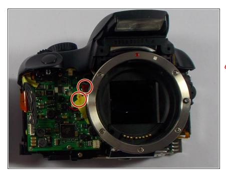
Remove the cable heads attached on the front side of the camera next to the lens mount.
