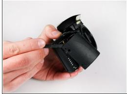
• Use the spudger tool to carefully pry the grip from the rest of the camera.
