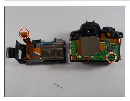
Once you have detached the back cover, use a pair of tweezers to lightly pull on strap found connecting the back cover to the camera.
