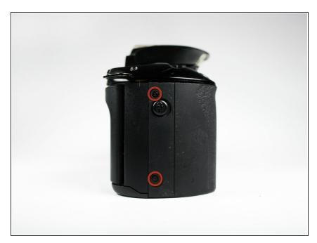
Remove the two 4.5mm (.18in) long black screws from the camera grip using a #00 Phillips screwdriver.
