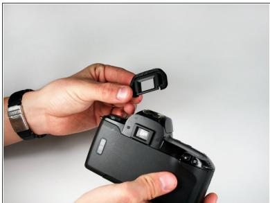
Grasp the eyepiece with your fingers and slide upwards to remove it.
