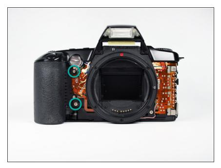
Remove the two 5mm (.20in) long silver screws securing the grip to the camera using a #00 Phillips screwdriver.
