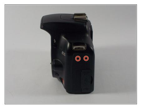
Remove the two 4.5mm (.18in) long black screws from the side cover using a #00 Phillips screwdriver.
