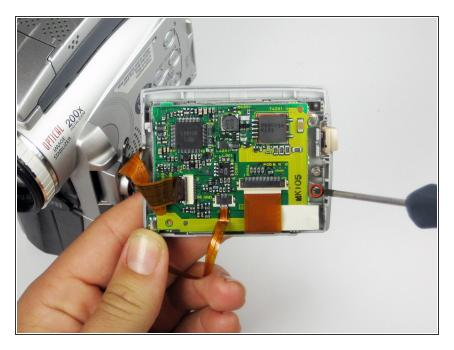
Remove the 4mm #00 Phillips screw connecting the LCD to the glass screen and lower casing.
