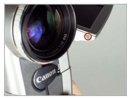
Remove the two 4mm #00 Phillips screws on the inside edge of the LCD casing. After removing the first screw you will have to rotate the screen 180 degrees to remove the second screw.
