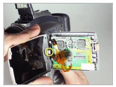
Disconnect the screen components from the main body of the camcorder by applying downward pressure near the circled hinge.
