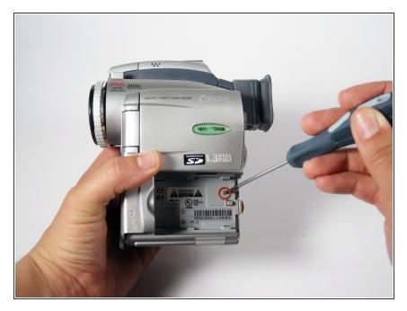
Remove the screw from inside the battery housing.
