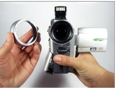
To remove the camcorder lens hood, twist the hood to counterclockwise and it will come loose, then pull towards you.
