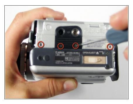
Remove the 4 Philips #00 4mm screws shown.
