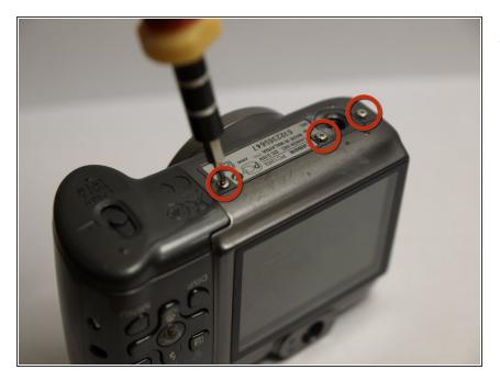
Remove the three screws located at the bottom of the camera using a magnetic screwdriver.
