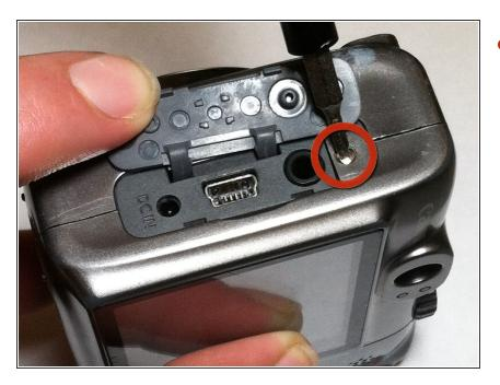
Remove the screw located under the rubber flap on the left side of the camera using a magnetic screwdriver.
