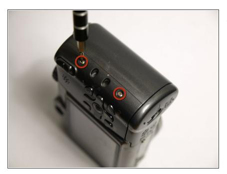
Remove the two screws located on the other side of the camera using a magnetic screwdriver
