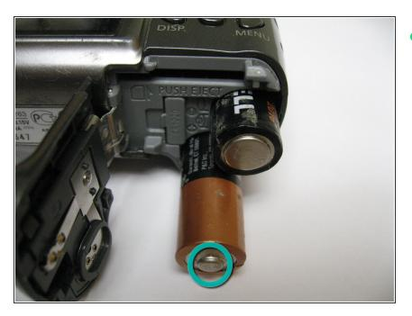
When replacing the AA batteries, verify they are oriented correctly by following the (+) and (-) signs on the camera.
