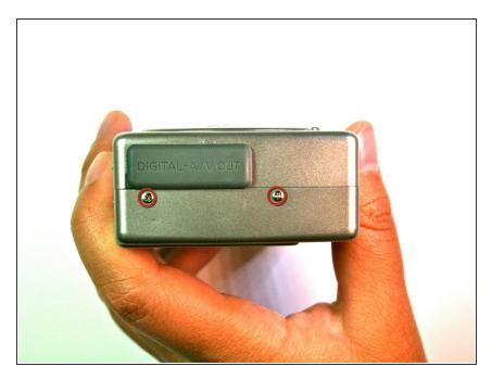
Remove the two 2.3mm screws from the right face of the camera.
