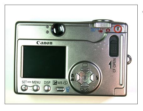
Remove the single 3.8mm screw from the back face of the camera.
