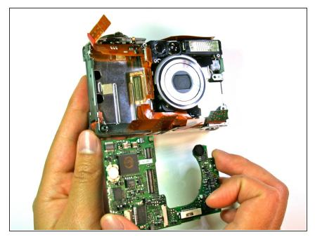
Carefully remove the motherboard from the main frame of the camera body.
