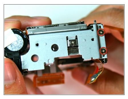
After completing the removal of the motherboard, remove the tripod mounting screws (3.4mm) on the left side
