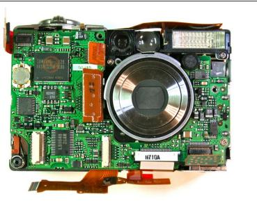
Remove the seven wire connections that connect to the motherboard.
