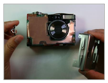
Remove the front face by sliding it off.
