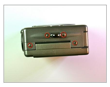
Remove the two 3.2mm screws (outside edge) and two 3.7mm screws (towards middle) from the left side of the camera body.
