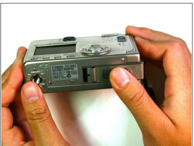
Slide grey latch to open the battery compartment.
