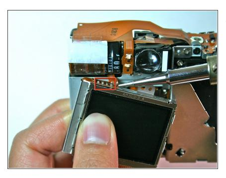
Unsolder the four points at the top of the screen with a soldering iron
