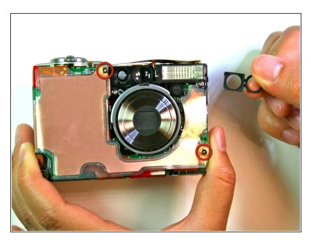
Remove the two 3.9mm screws that retain the laminated cooper sheet.
