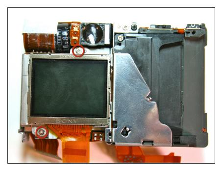
Remove the 2.1mm screws from the bottom and top of the screen connecting it to the housing plate
