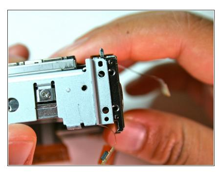
Carefully pry the left side of the housing plate from the bottom of the tripod mounting plate, releasing it from the two alignment pegs next to the screws
