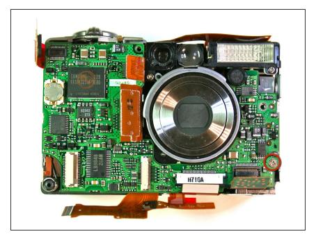
Remove the single 3.8mm screw that is on the motherboard.
