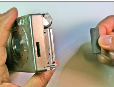
Remove the rubber digital a/v out cap by sliding it out of the groove on the front plate.
