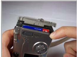
Push down on the black square button next to the memory card slot. This will release the memory card from the slot.
