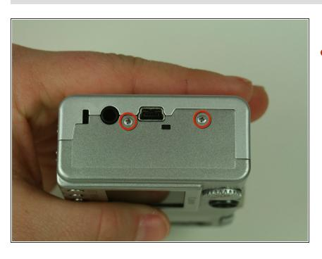
On the side of the camera, remove the two 4.75 mm screws that sit near the USB digital terminal.
