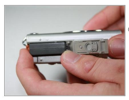
Grasp battery and fully pull out of slot
