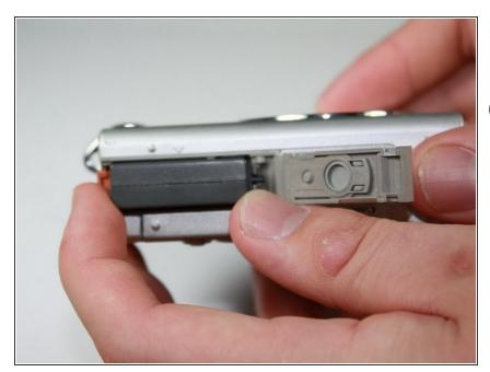
Grasp battery and fully pull out of slot
