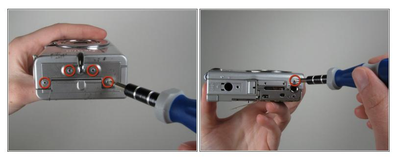
Unscrew the four Philips screws from the side of the casing and one screw from the bottom using a #0 Phillips screwdriver.
