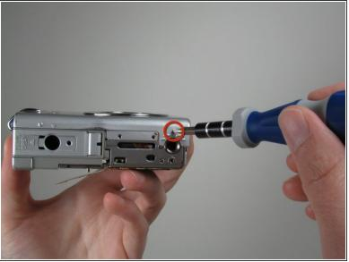
Unscrew the four Philips screws from the side of the casing and one screw from the bottom using a #0 Phillips screwdriver.
