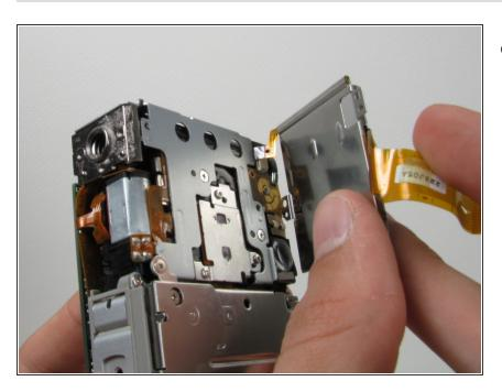
Lift the LCD away from the rest of the camera.
