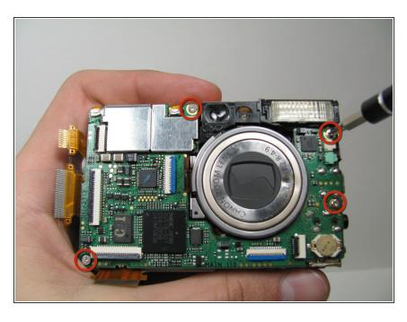
Unscrew the four Phillips screws using a #0 Phillips screwdriver.
