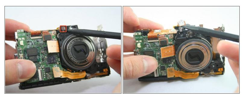
• Use spudger to carefully lift the LED light off the upper-left corner of the lens.
