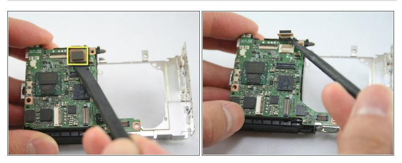
• Using the spudger, disconnect the ribbon cable located on the top of the logic board.
