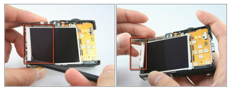
• Use the spudger to remove the L-shaped bar from the left-side of the LCD screen.
