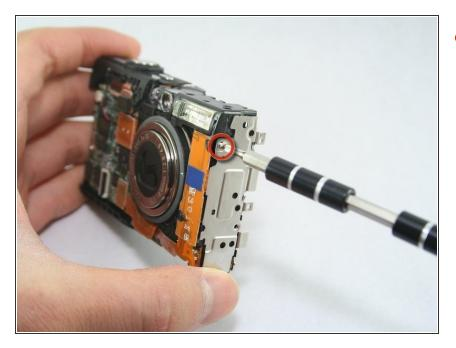
• Remove the screw located on the side of the camera (0.072 in).
