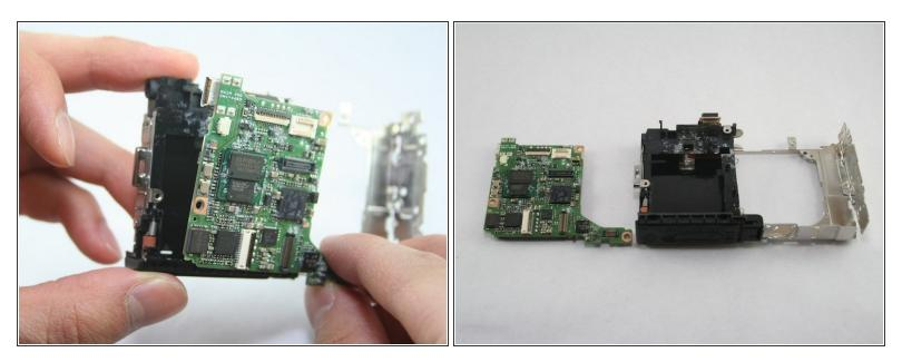
• The logic board may now be removed from the frame.
