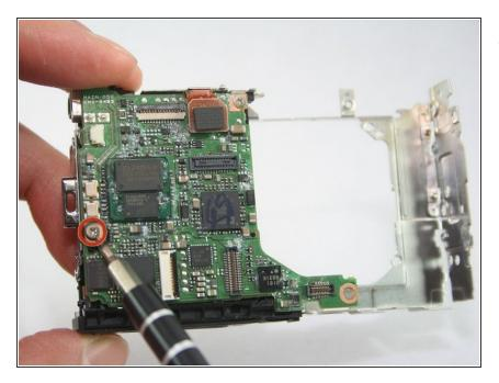
• Remove screw (0.102 in) from the left side of the logic board.
