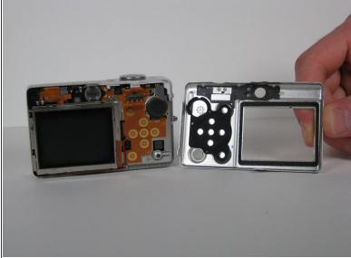
Use your fingers to carefully pry off the back casing from the camera assembly. Casing should lift straight off.
