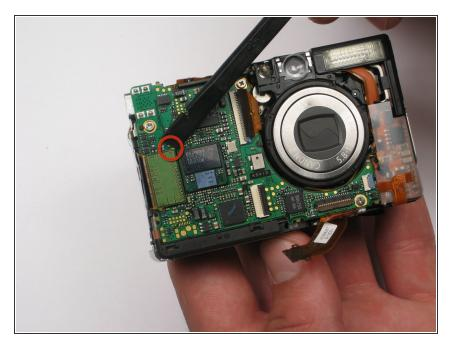
Lift up the large green flap by using the spudger to pry up top right yellow edge.
