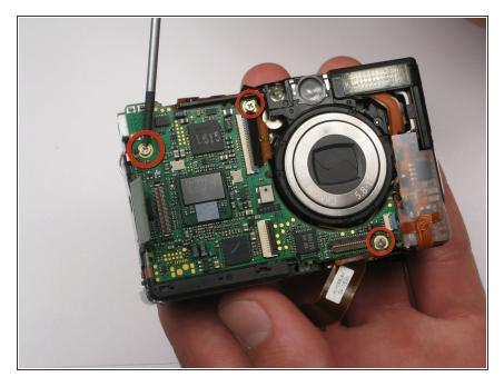
Use the screwdriver to remove the three screws on the logic board.
