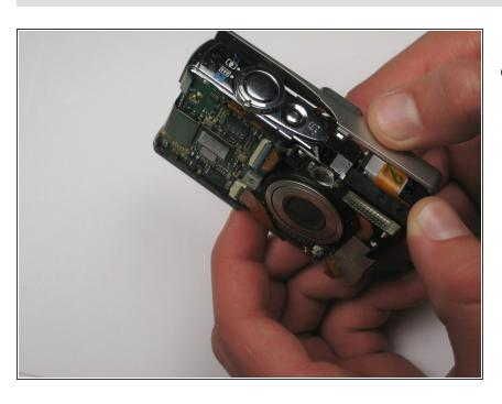
Take hold of the inside of the camera, and gently pull away from the back casing.
