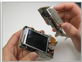
Now the camera body is loose. gently lift the rear of the case to remove it from the camera.
