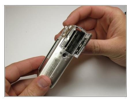
In preparation for disassembly, the battery and SD Card need to be removed from the camera. You can access both the battery and the SD card through the door on the bottom of the camera.
