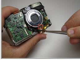
• One by one, detach the three ribbon cables from their ports.
