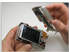
Now the camera body is loose. gently lift the rear of the case to remove it from the camera.
