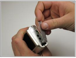
On the left side of the camera, there are two .085 inch screws. Remove these, then lift the plate from the camera.
