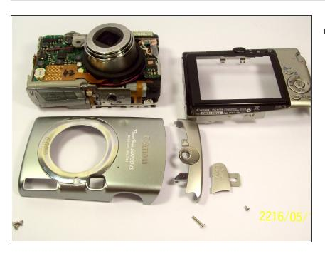
Remove the front back and side casings from the camera.
