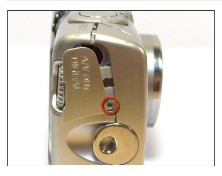
Remove the screws on the left of the camera underneath the "A/V out Digital" cover flap.
