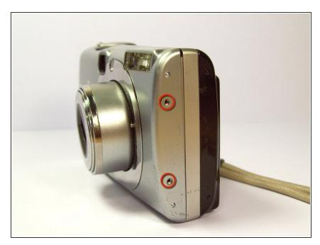
Remove the screws on the right side of the camera.
