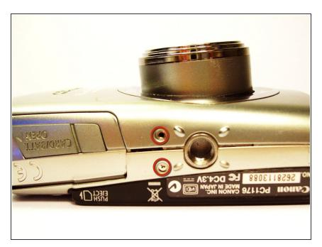
Remove the screws on the bottom of the camera using a 00 Philip's head screw driver
