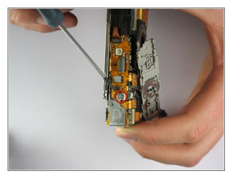
Remove screw attaching the Mini USB Cover to the top of the camera body.
