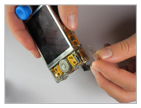
Remove Mini USB Cover, by pulling it away from the camera body.
