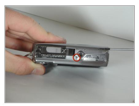
Remove one 2.25mm screw on the bottom.
