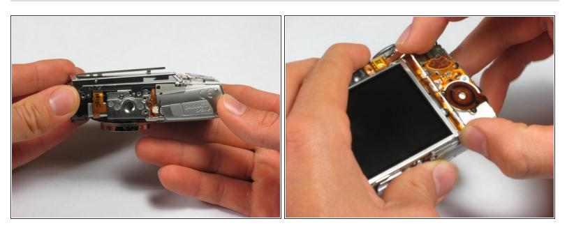
• Remove the two metal frames that hold the LCD panel in place.
