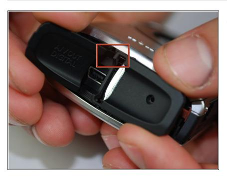
Carefully unhook the "A/V OUT DIGITAL" cover from the hinge.
