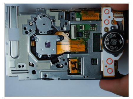
The metal back plate can now be removed. All that is holding it on at this point are pins and wires connected to the logic board.
