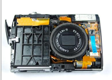
Pull the front cover from the camera by using gentle upward pressure.
