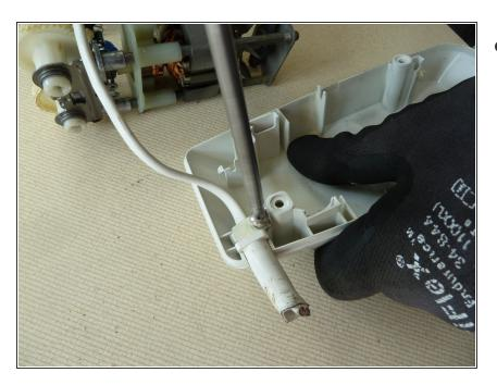
• Unscrew the power supply cable.
