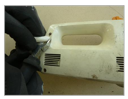
• Cut the power cable. Dispose of the plug separately (mixed waste).
