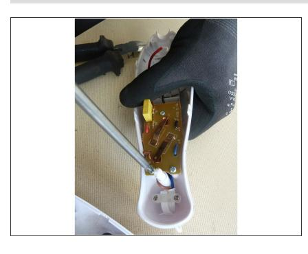
Unscrew the printed wiring board (PWB).
