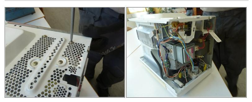
Remove the remaining screws on the back cover.
