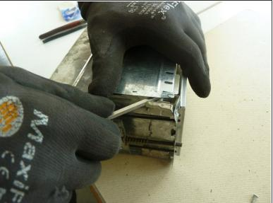
Remove the cover of the heating unit.
