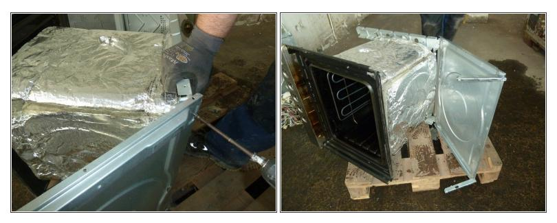
• Unscrew and remove the bottom.
