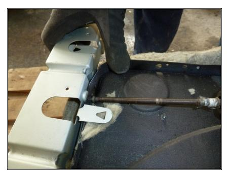
• Remove the metal rails that held the insulation wool.
