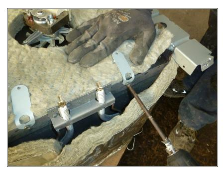
• Unscrew and remove the fixtures insulation.
