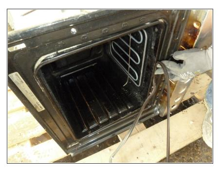
• Peel off the rubber sealing.
