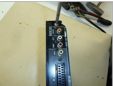
Remove all the screws from the side and the back of the casing.
