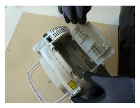
Remove the batteries and the battery cover.
