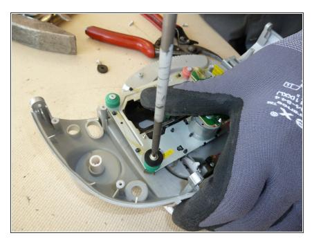
Unscrew and remove the tape deck device.
