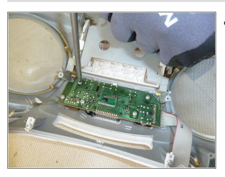
Unscrew and remove the PWB.
