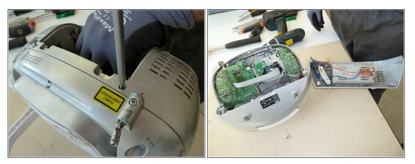
Remove the screws from the back of the case and take it off.
