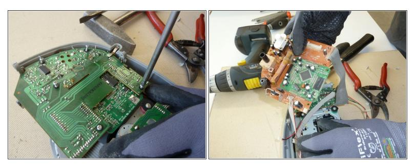
Unscrew and remove the PWB.
