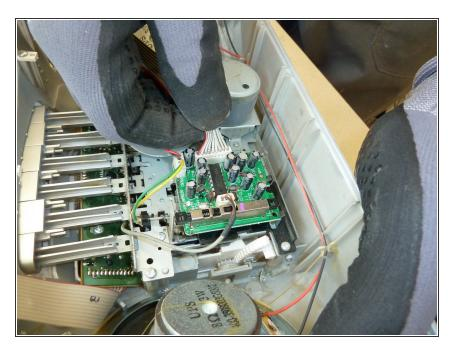
Unclip the wires from the PWB.
