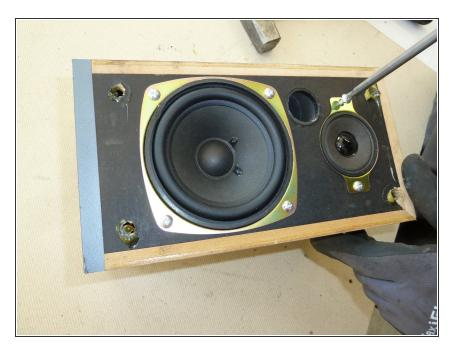
Remove the screws from the front of the speakers.
