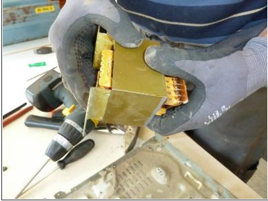
Unscrew and remove the coil.
