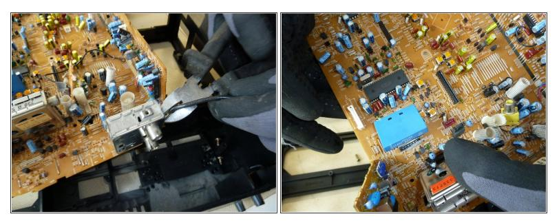
• Cut the wires and remove the delay line.
