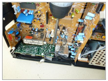
• Unscrew and remove the PWB.
