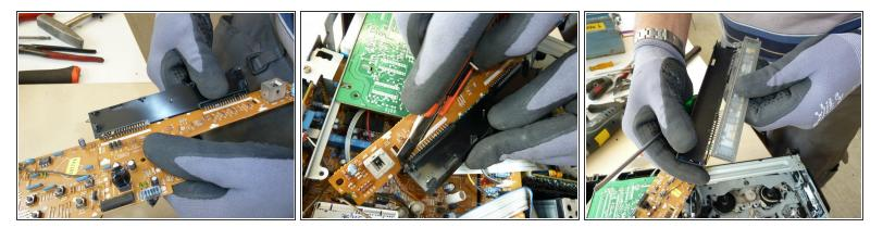
• Bend the display, cut its connectors and remove it.
