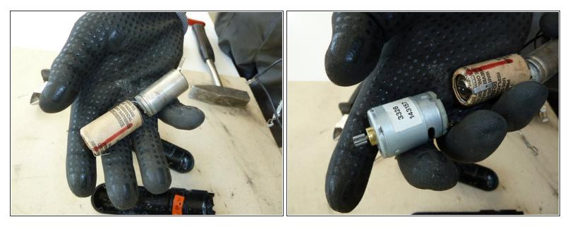
Remove the battery, the motor and the capacitor.
