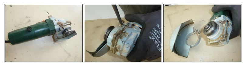
• Unscrew and remove the protection cover.
