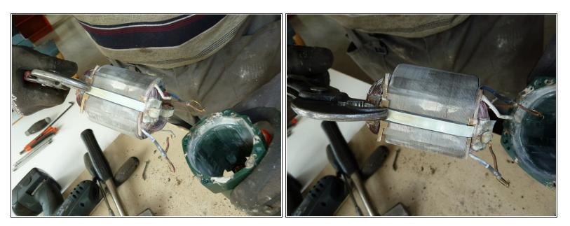
• Remove the stator.
