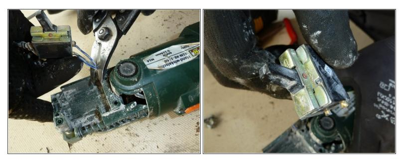
• Cut the wires of the power switch and remove it.
