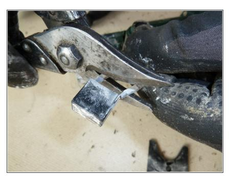
• Cut off the wires of the capacitor and remove it.
