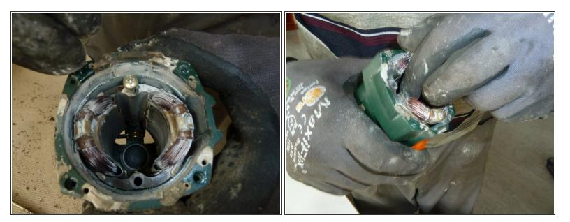
• Remove the stator.
