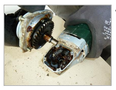
• Lift off and remove the gear.
