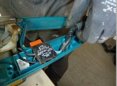
Unscrew and remove the power cable.
