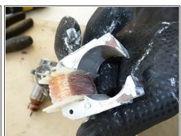
Remove the motor and the motor coil.
