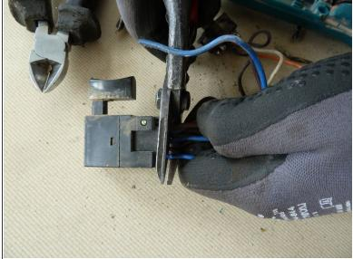
Remove the switch and cut its cables.
