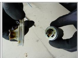
Unscrew and remove the motor.
