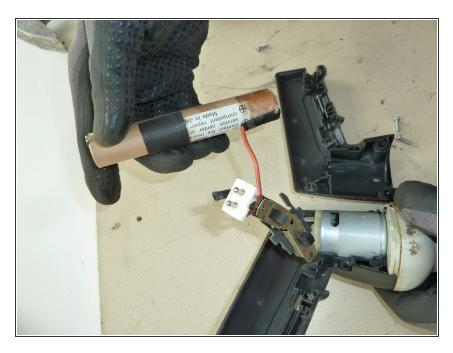
Remove the batteries.
