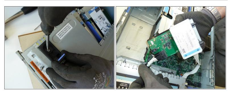
Unscrew and remove the electronic parts.
