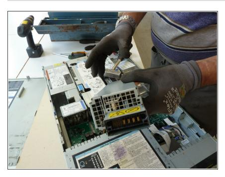
Remove the power supply element.
