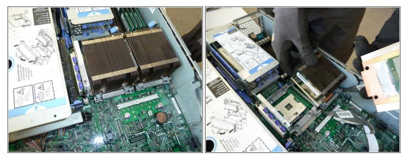
Remove the aluminium heat sinks.
