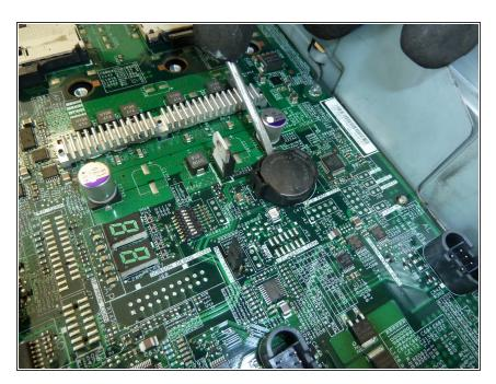
Pry out the cmos battery.
