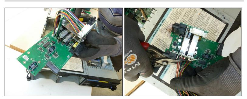
Cut the wires off the electronics.
