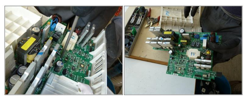
• Unscrew and remove the PWB.
