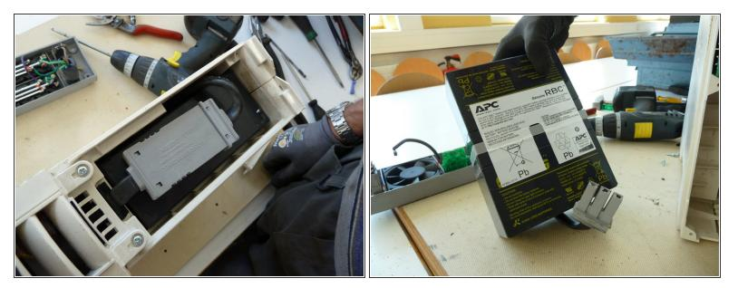
• Remove the lead batteries.
