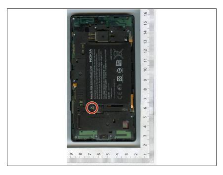
Loose one T4 screw to remove the battery connector strap
