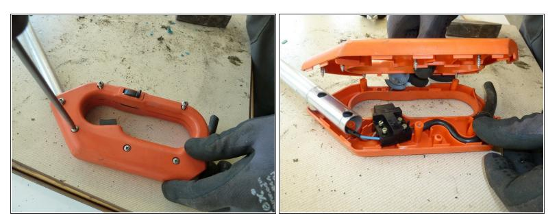
At the end of the handle, unscrew and open the plastic handle.
