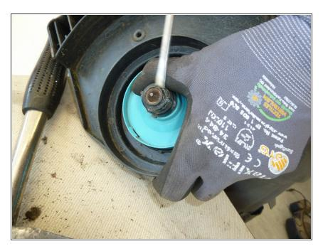
Flip the trimmer over to remove the drive shaft.
