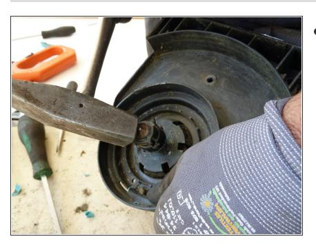
Remove the drive shaft by hitting it with a hammer.
