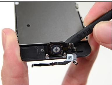
Peel the home button the rest of the way off of the display by prying gently with a spudger.
